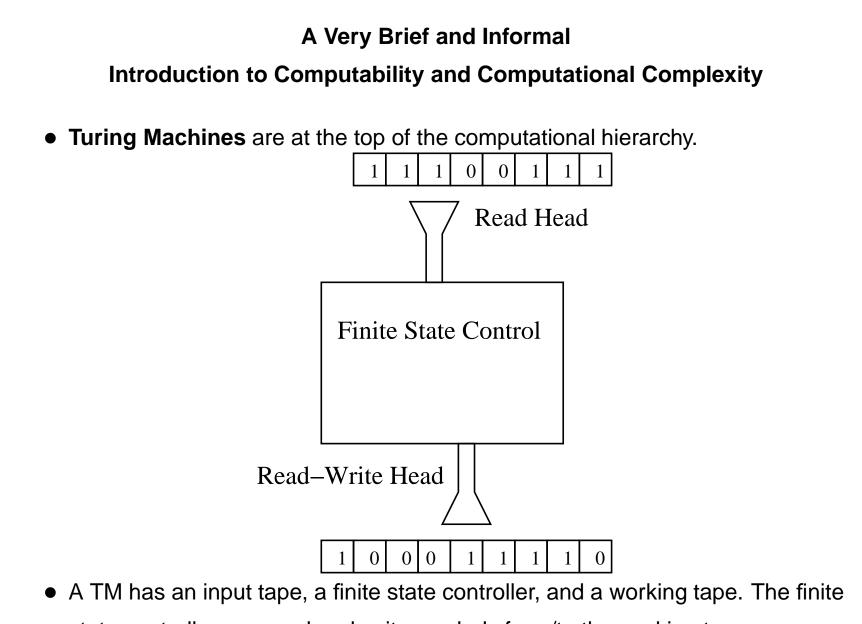
state controller can read and write symbols from/to the working tape.
